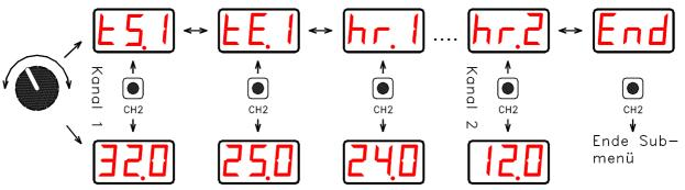
It is to be noted that the programmed starting value always has to be greater than the end value. If the values are not programmed properly (tS.. < = tE..), the timer cannot be started. Control continues as before according to the **tE..** value.
