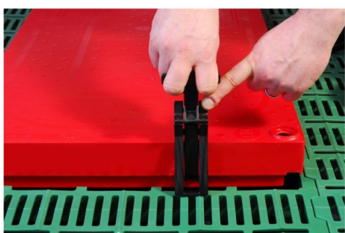
3. lift the panel with the tool
